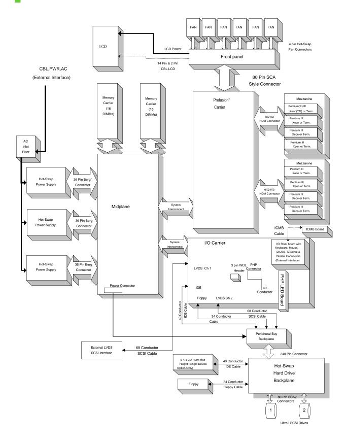
Figure 4-1: OCPRF100 Server System Interconnect Diagram
